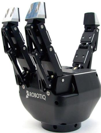
Figure 5. 3-finger gripper from ROBOTIQ.<sup>31</sup>
