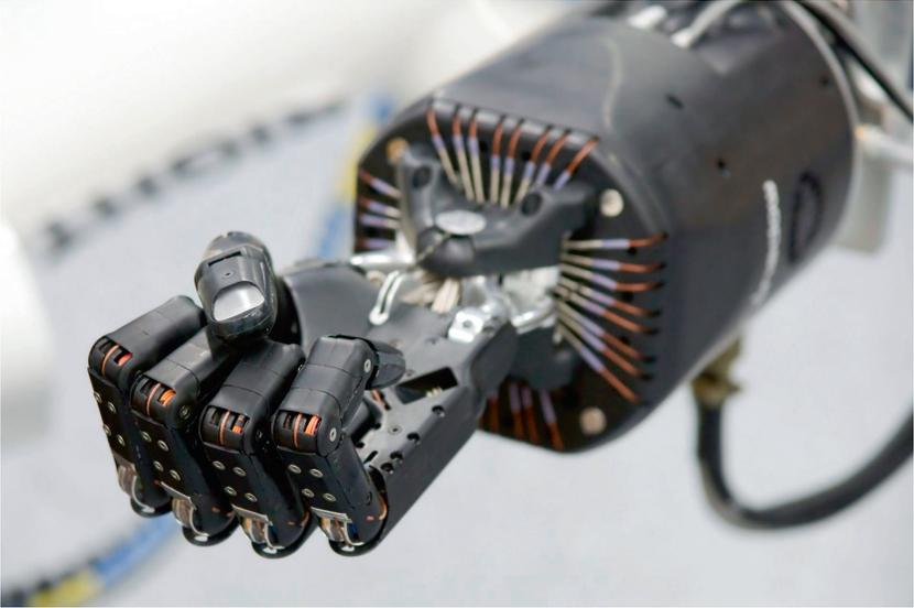
Figure 6. 5-finger gripper.<sup>32</sup>
