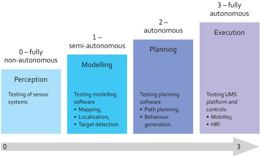
Figure 3. NCAP levels within generic UMS architecture model<sup>13</sup>.
