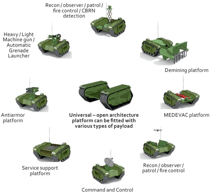
**Figure 2. Inventory of vehicle -transportable/self-transportable unmanned systems**
