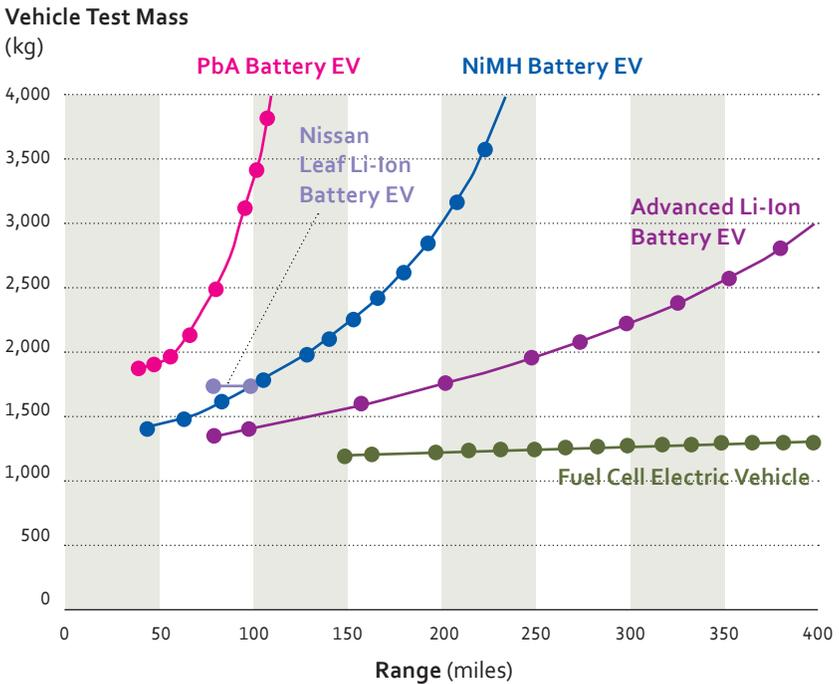
Figure 2. Vehicle test mass\* versus driving range for different batteries.<sup>8</sup>
