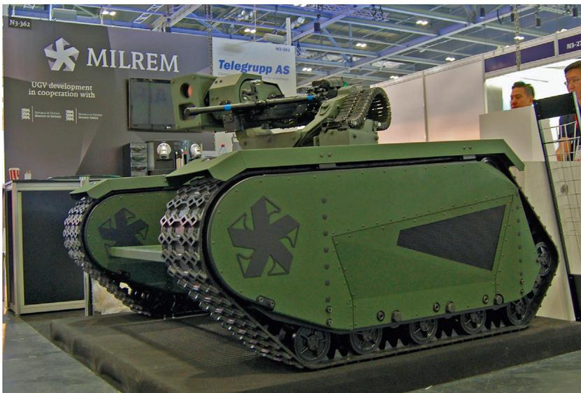
Figure 3. The UGV from MILREM with firearm system mounted.<sup>12</sup>
