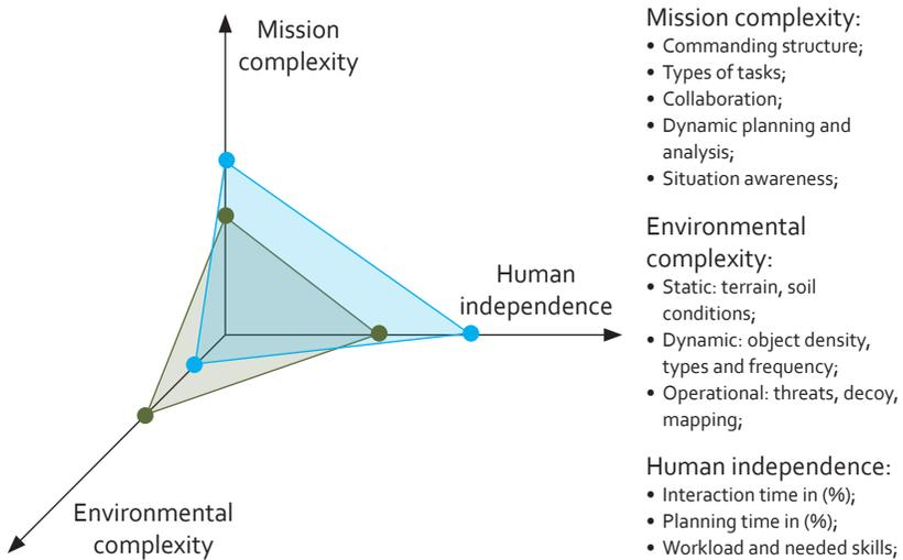
Figure 1. ALFUS scoring axes and parameter examples<sup>6</sup>.
