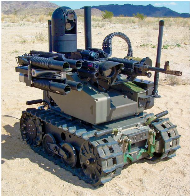
**Figure 3. MAARS (Modular Advanced Armed Robotic System)**
