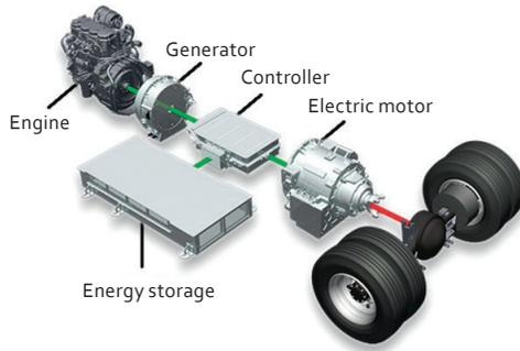
**Figure 1: Integration the series hybrid into available vehicle**
